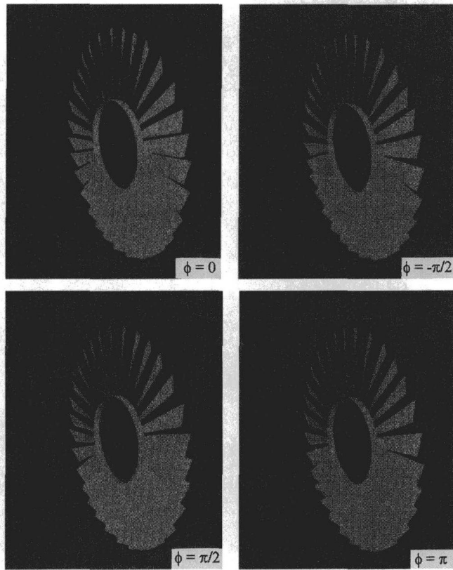
Fig. 11 Schematic of Chi_B cascade bending vibration at \beta_r = 72 deg
